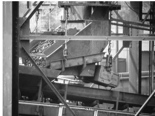
Large-capacity Jeffrey feeders blending stone.
