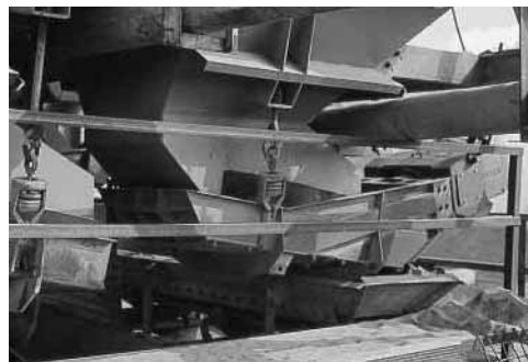
Group of feeders blending stone to meet highway specifications and fitted with dust seals.
