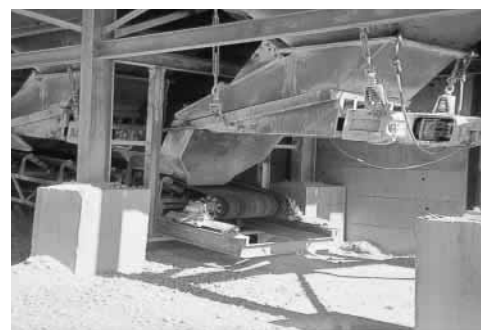
Model HP300 feeder continuously feeding to belt conveyor.
