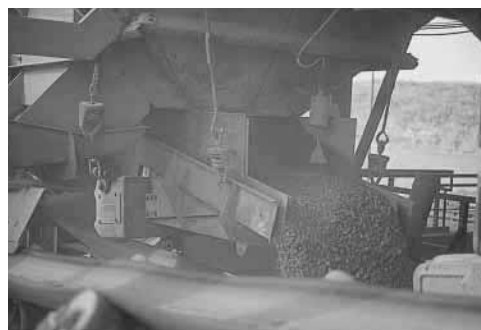
Stone blending is controlled by Jeffrey feeders.
