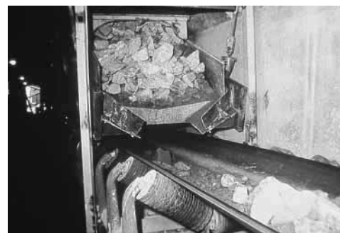
Model HP400 feeds 700 TPH of stone. Note belt deflectors on deck, a Jeffrey first.
