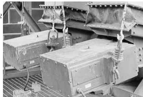
Group of feeders blending stone to meet highway specifications and fitted with dust seals.
